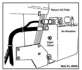
The oil level sight glass is located on the back of the reservoir. The oil level should be even with the sight glass and checked with the cutter unit in the transport position. The oil temperature should not exceed 180 deg.F.
